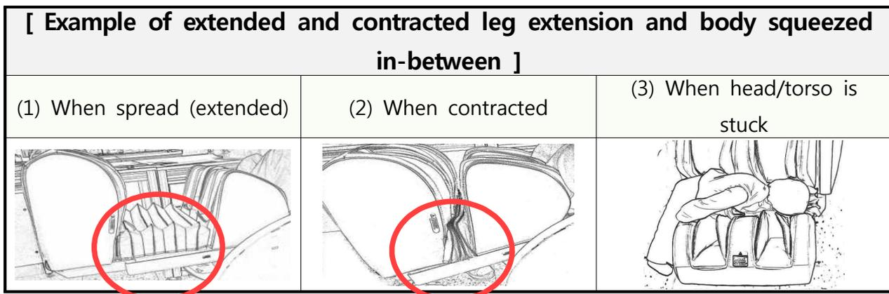
The **leg extension widens or contracts** when measuring body type before massaging or operating specific massage mode. **During this process, infants can be squeezed inside**. When the massage chair fails to detect and contracts, significant pressure is given to the body.
